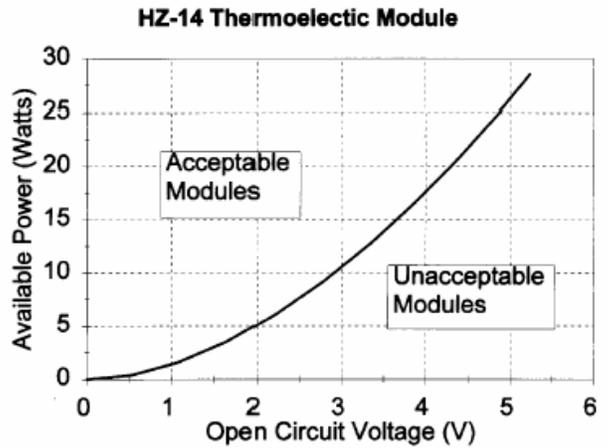
Figure 8. Power vs Open Circuit Voltage
