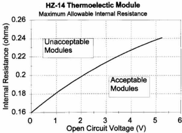
**Figure 9. Internal Resistance vs Open Circuit Voltage**
