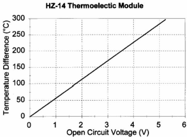
Figure 7.  $\Delta T$  vs Open Circuit Voltage
