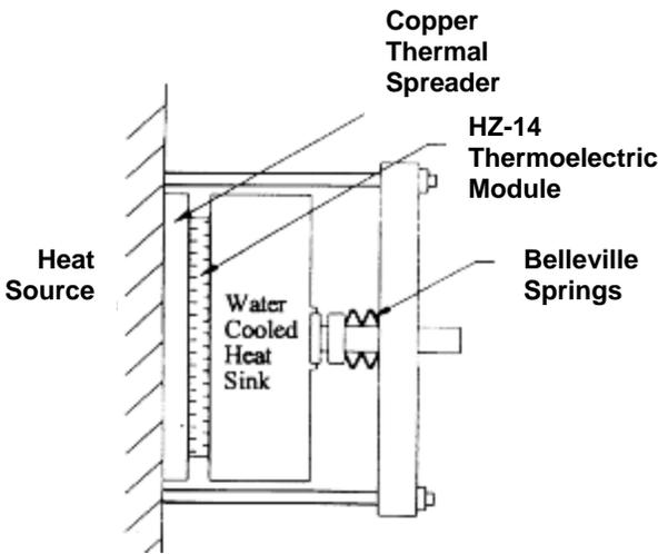
Figure 2. Module Pressure System
