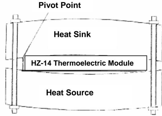
Figure 3. Bowing of Heat Sink/Source
