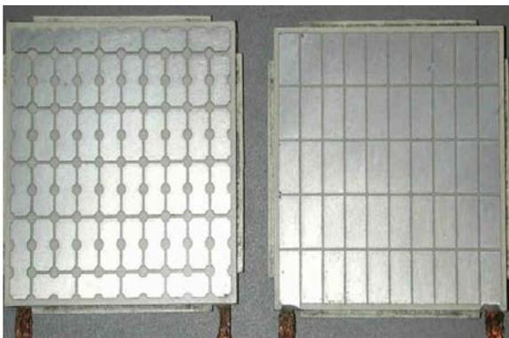
**Figure 1 – H Z-14 Thermoelectric Module Showing the Cold Side (right). The hot side (left) shows dots of the “egg crate” material.**
